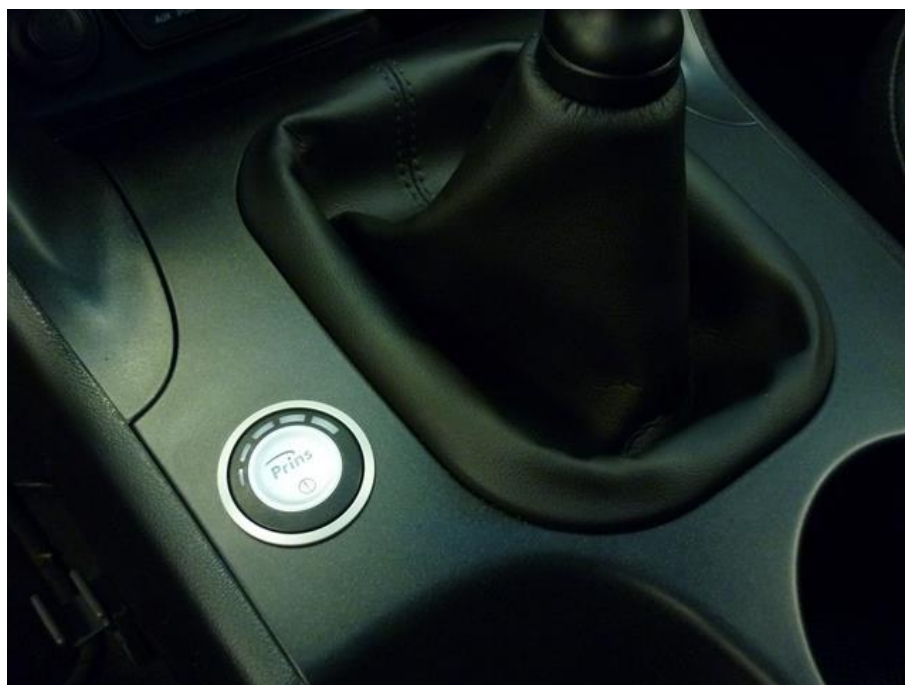
( Drill Ø32 mm, Forstner drill, install switch with cup holder )
