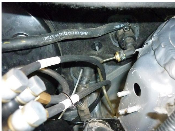
Connect the fuel hoses to tank
