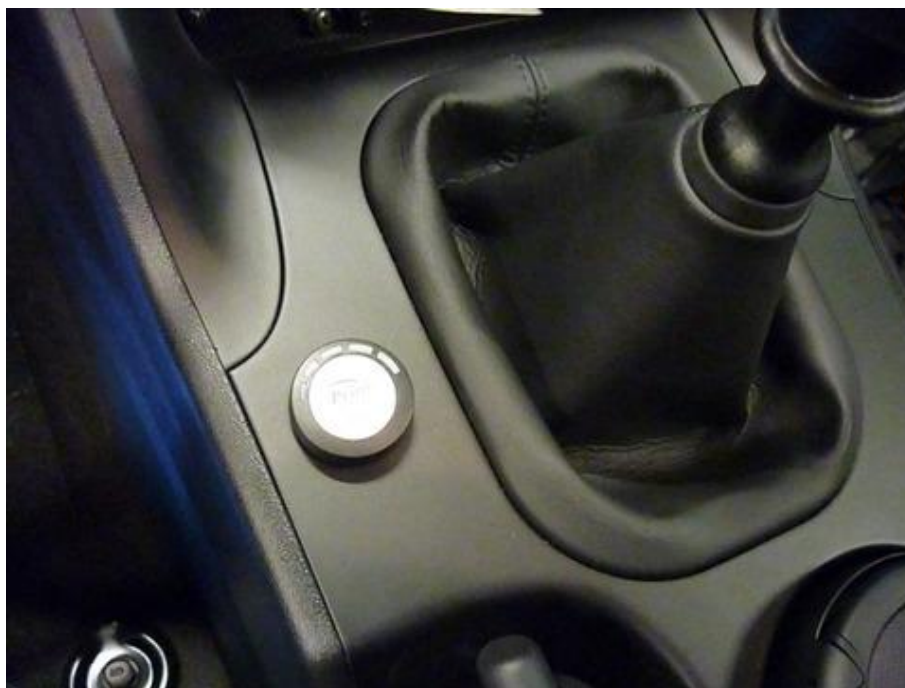
Drill Ø8.3mm, mount the switch
