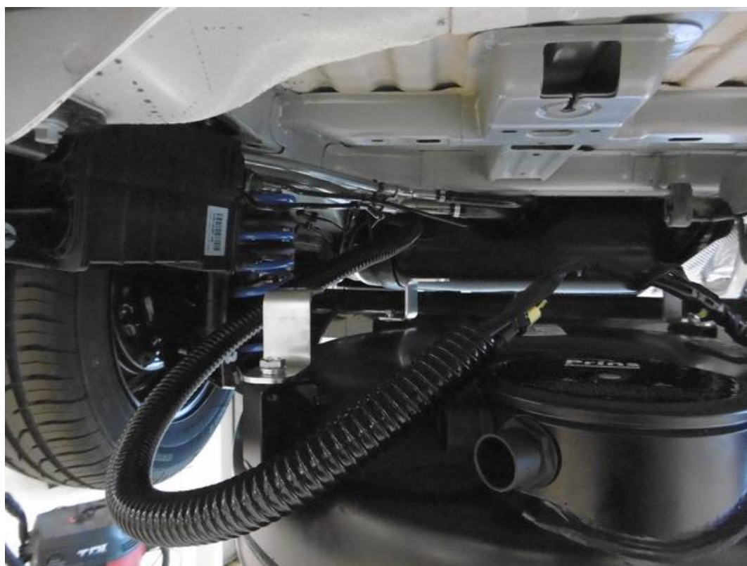
130cm ventilation pipe
