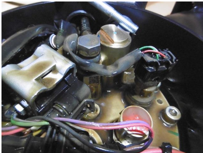
Spray with clear body coat when fuel lines are connected.
