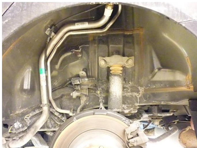
Remove inner mud guard
