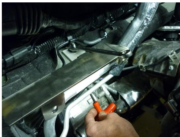
Use an Allen key and 10mm wrench to tighten the bracket
