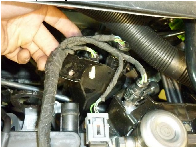
Tect connector: under HPPump housing:
