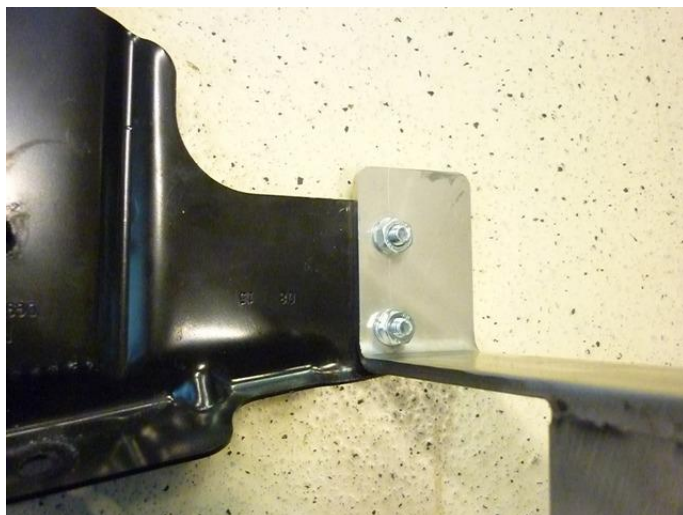
Mount sub bracket and re-install ECU support bracket.
