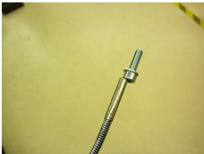
Use a flex magnet to install the Allen bolt
