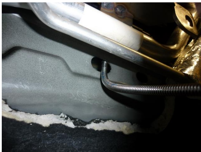
Use a flex magnet to install the Allen bolt
