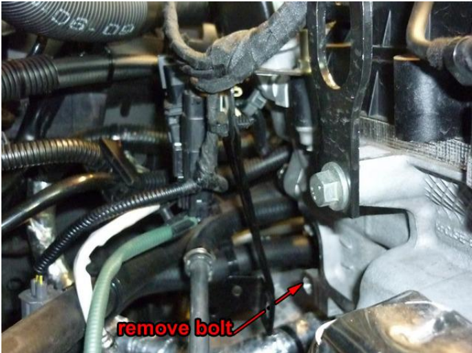
Tect connector: under HPPump housing:
