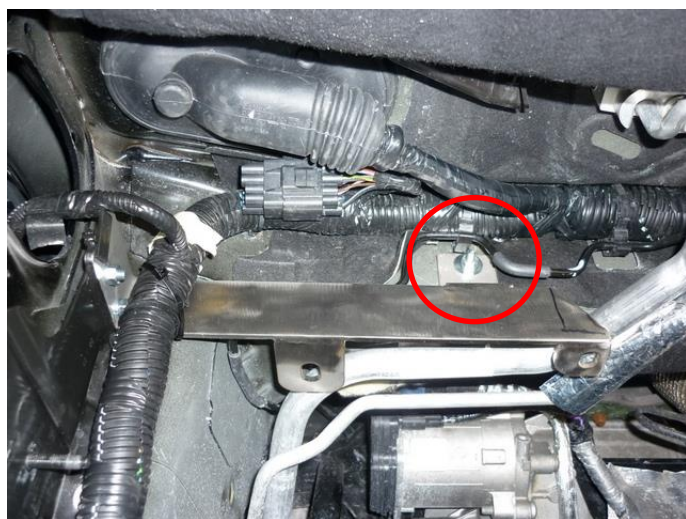
Use an Allen key and 10mm wrench to tighten the bracket
