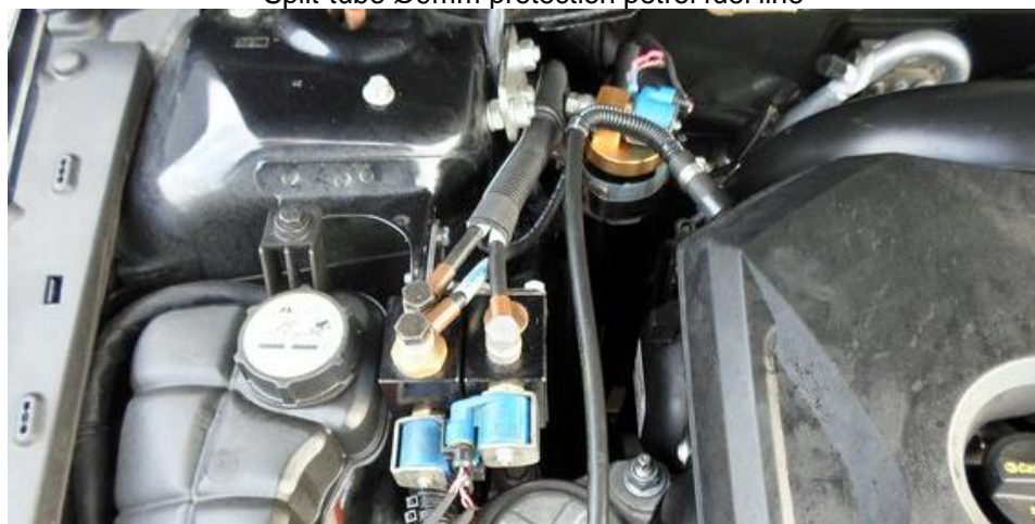
Split-tube Ø9mm protection petrol fuel line
