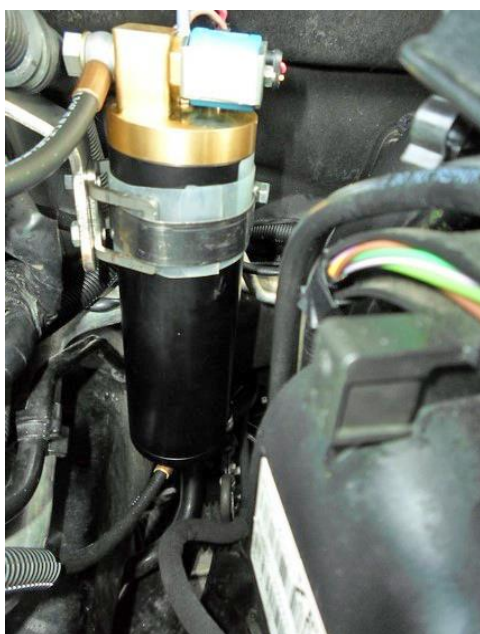
Split-tube Ø9mm protection petrol fuel line
