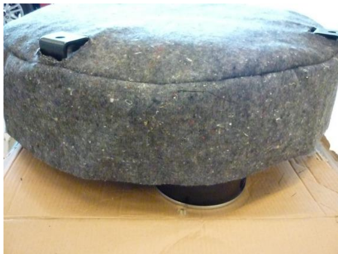
Install insulation cover
