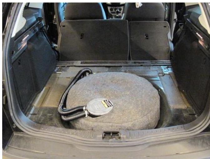
Place tank, drill 4 x Ø11mm
