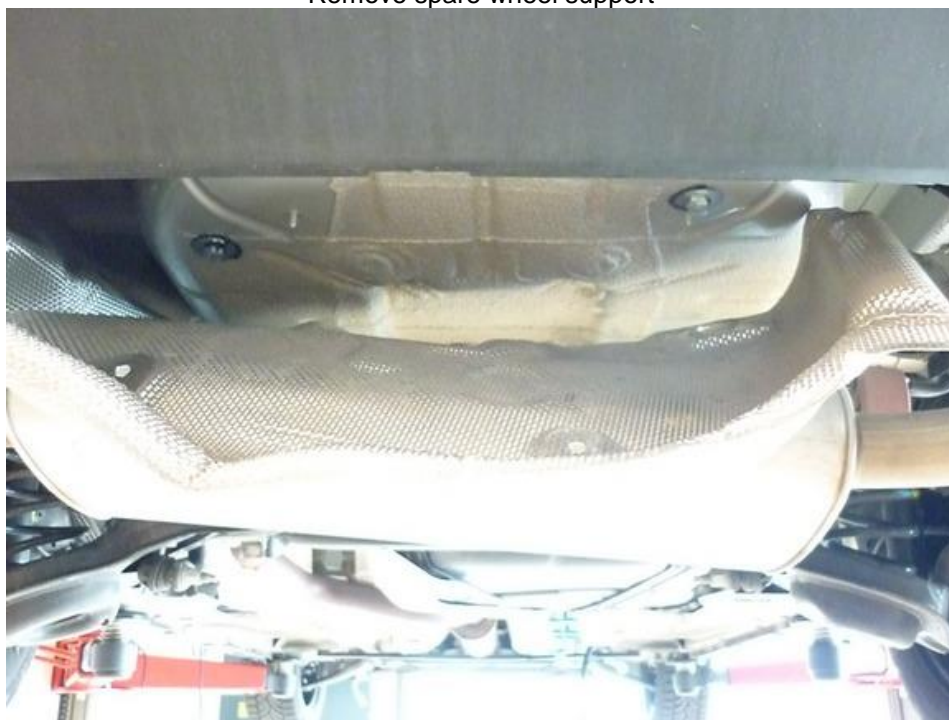
Loosen heat shield
