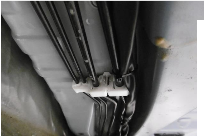
Use heat reflecting foil sticker ( wrap fuel lines and wiring )
