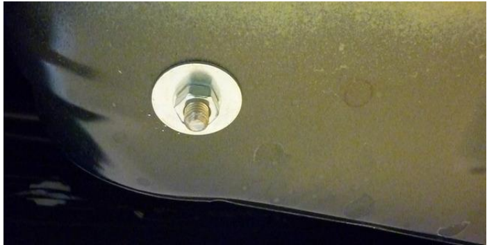
Punch the holes and drill from underside Ø8.2mm
