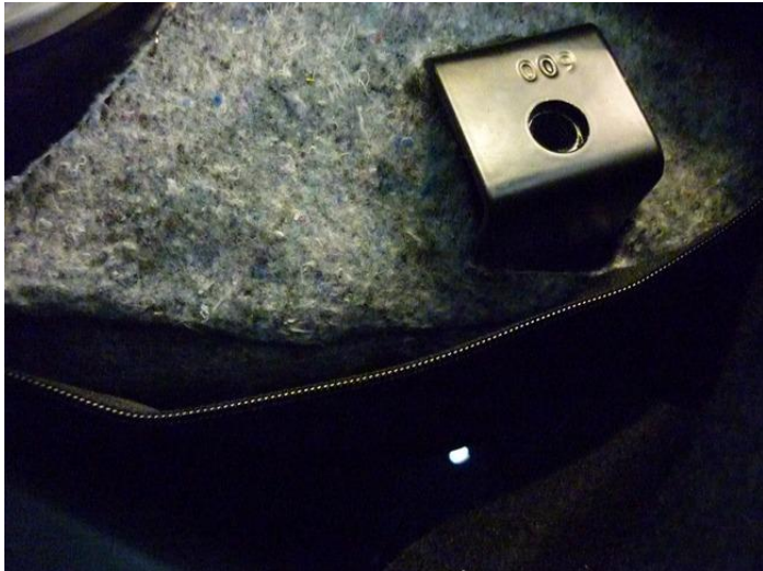
Punch the holes and drill from underside Ø8.2mm
