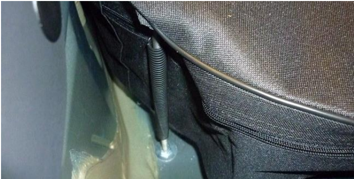
Punch the holes and drill from underside Ø8.2mm
