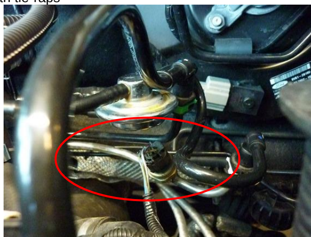
Original hose connected to the boost pump inlet ( petrol supply line with Low Pressure petrol sensor )
