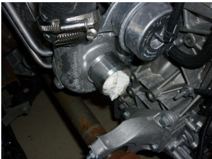
Remove inlet pipes and block hose inlets and turbo inlet.
