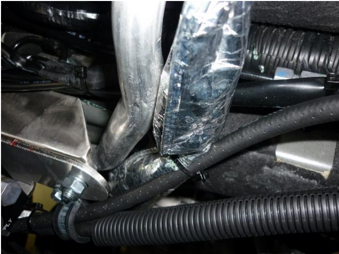
Secure fuel hose with cable tie to the hose clamp.
