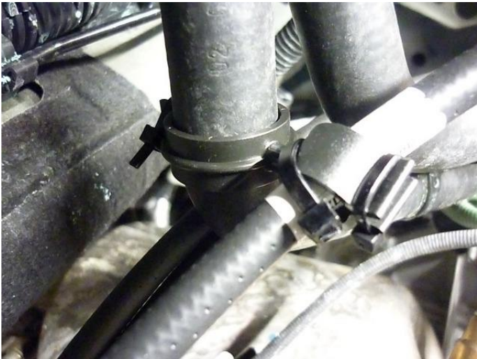
Secure fuel hose with cable tie to the hose clamp.
