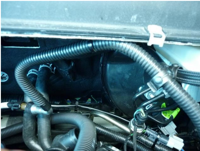
Secure fuel hose with cable tie to the hose clamp.
