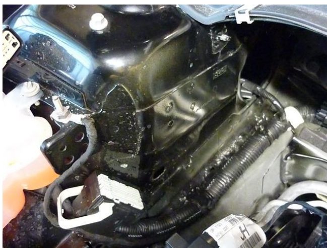
Remove petrol ecu with support bracket.
