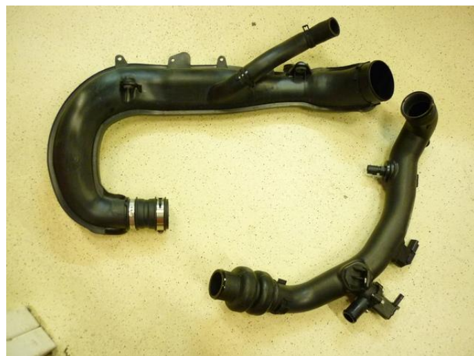
Remove inlet pipes and block hose inlets and turbo inlet.
