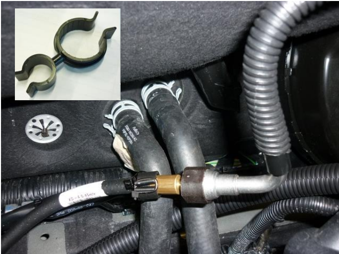
Secure fuel hose with cable tie to the hose clamp.
