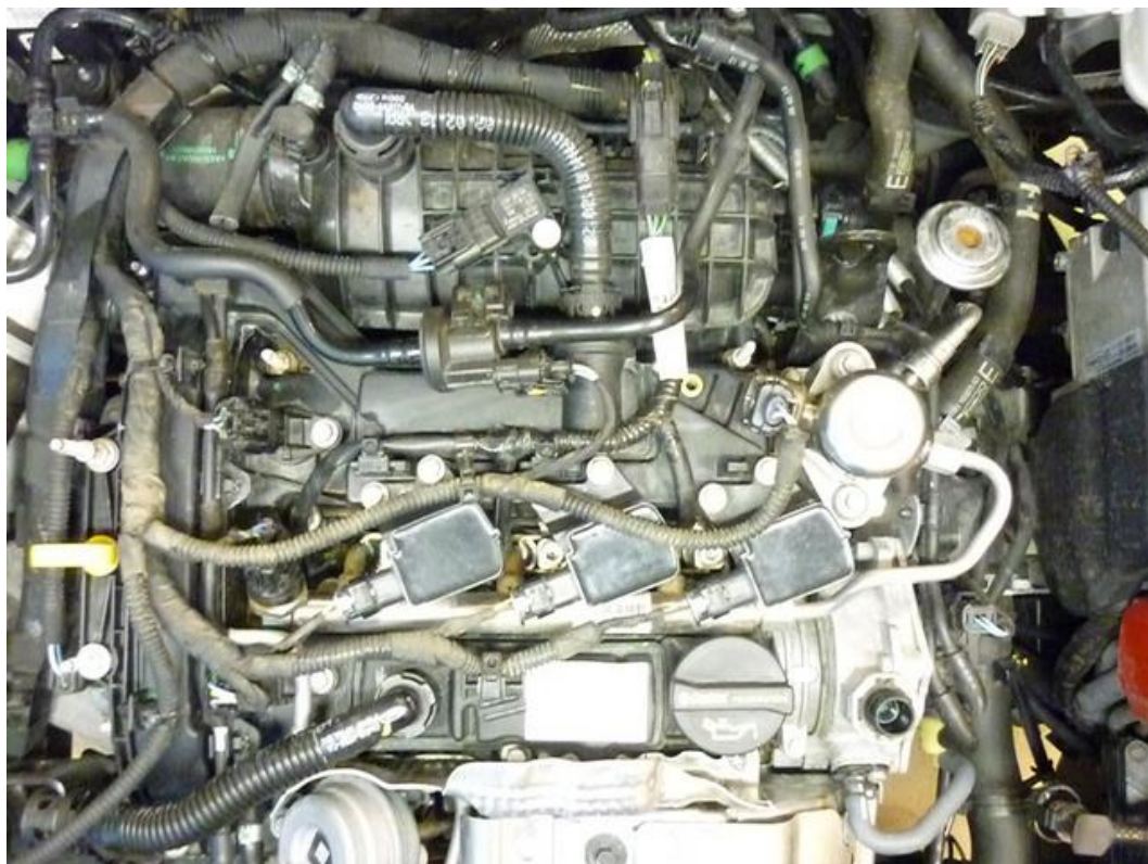
Removed air filter box and inlet pipe ( turbo -> air box )
