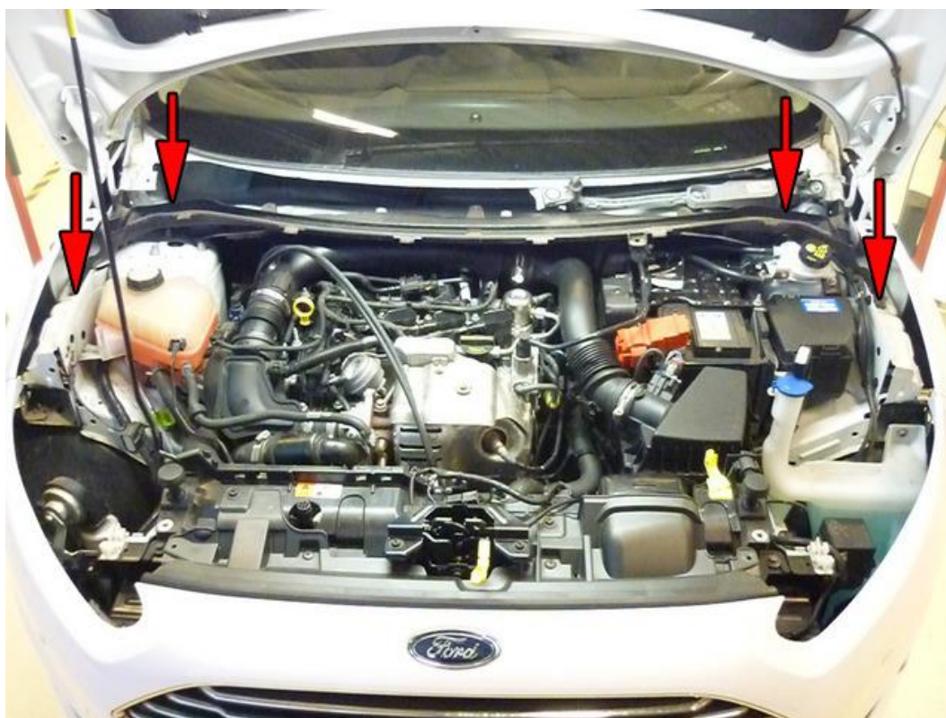
Remove wipers, cowl panel and fire wall panel ( 4 screws )
