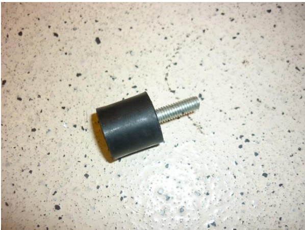
Screw two vibration dampers (25x15) on the M6 studs.
