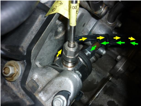
Lines from FSU and FRU unit to High pressure pump.
