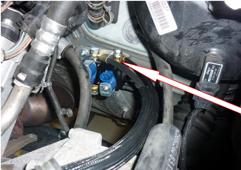
Screw two vibration dampers (25x15) on the M6 studs.
