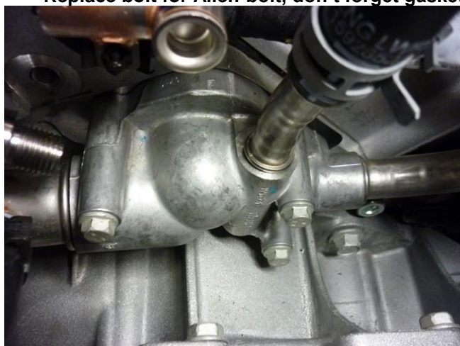
Mount the thermostat housing with a NEW GASKET refill engine coolant
