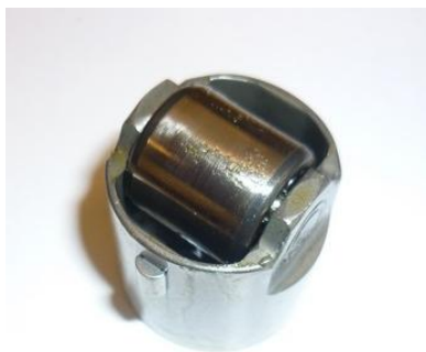
Check Roller Tappet before installation HPP pump
