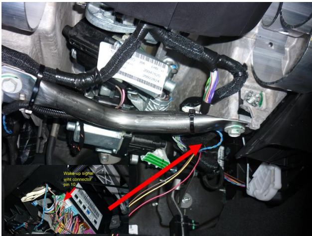
The module is mounted above the accelerator pedal.
