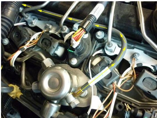
Return hose to FRU pressure sensor.
