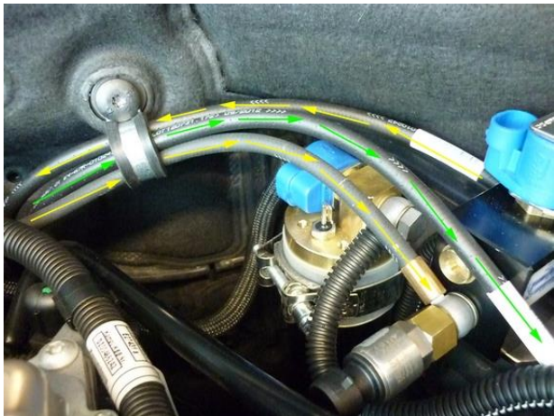
Return hose to FRU pressure sensor.
