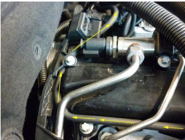
Return hose to FRU pressure sensor.
