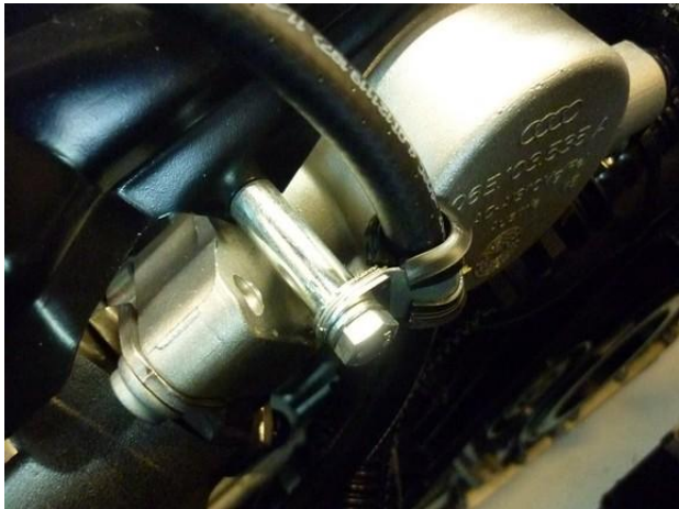
70 cm HPP fuel hose supply, clamp on 18cm.
