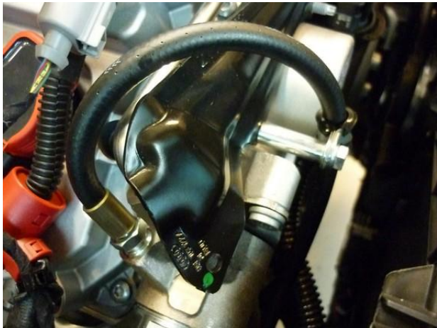
70 cm HPP fuel hose supply, clamp on 18cm.
