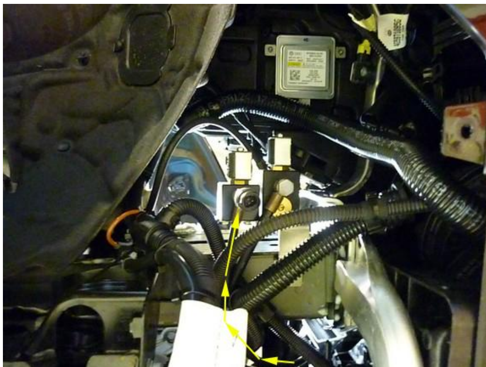
Return hose, banjo connection into sensor M10 hole
