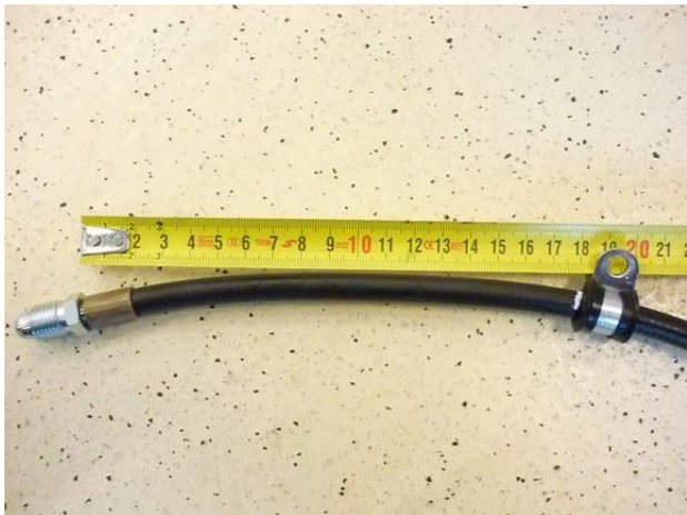
70 cm HPP fuel hose supply, clamp on 18cm.
