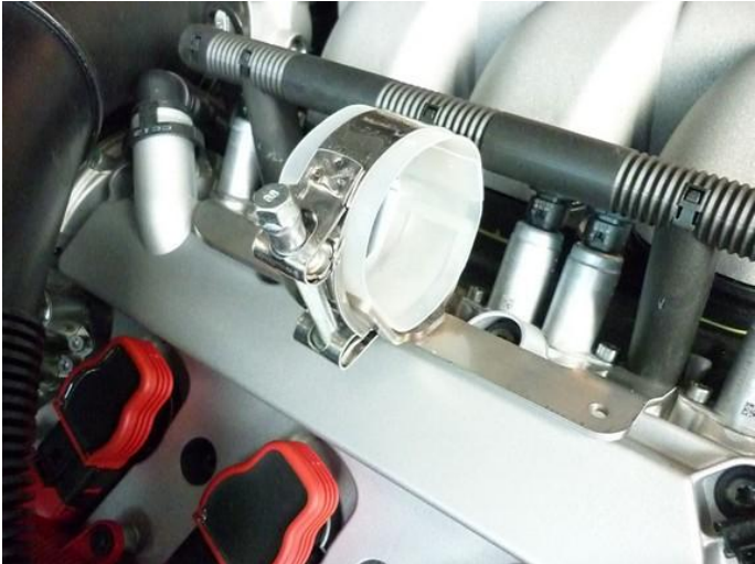
Mounting points bracket : underneath wiring loom pillars, use original bolts
