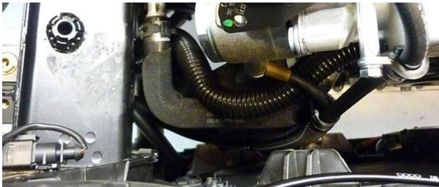
Return hose, banjo connection into sensor M10 hole
