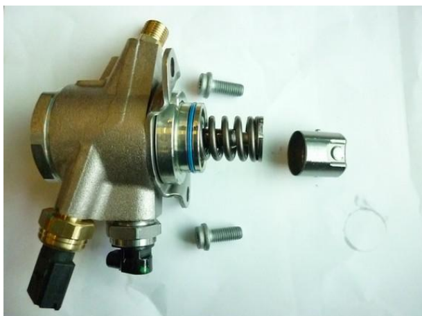
Roller tappet can slide out of housing !!
