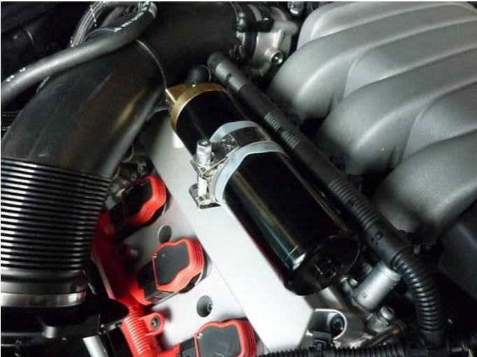
Mounting points bracket : underneath wiring loom pillars, use original bolts
