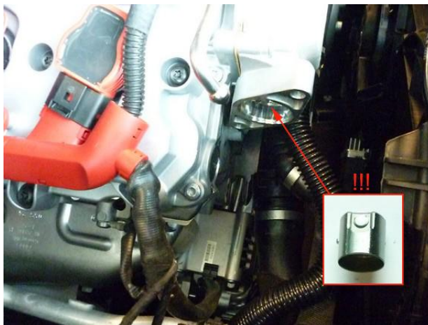
Roller tappet can slide out of housing !!
