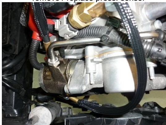
Install return hose into sensor connection with banjo bolt and two bonded seals.
