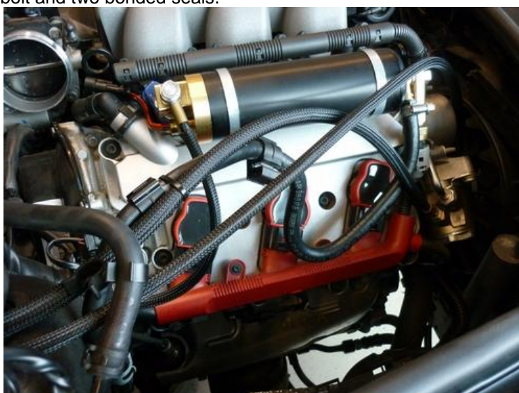
Install return hose into sensor connection with banjo bolt and two bonded seals.
