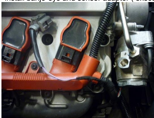
Split pressure-sensor wiring from loom.
