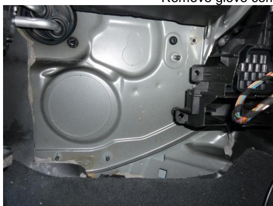
Remove glove compartment and foam
