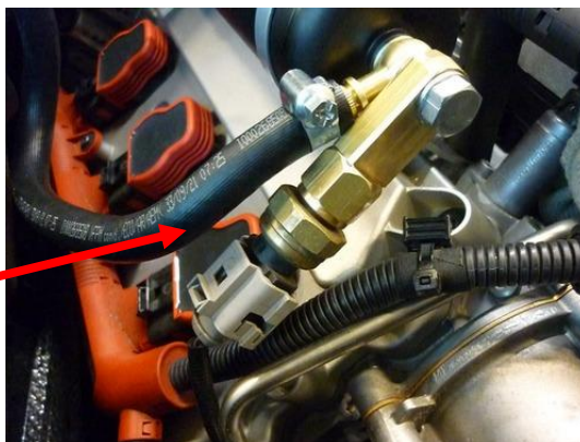
install banjo-eye and sensor adaptor ( 3xseal)
