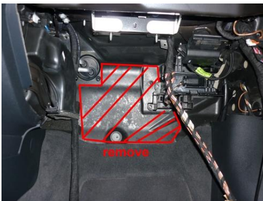
Remove glove compartment and foam
