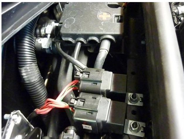
Mount relays onto threaded rods.
