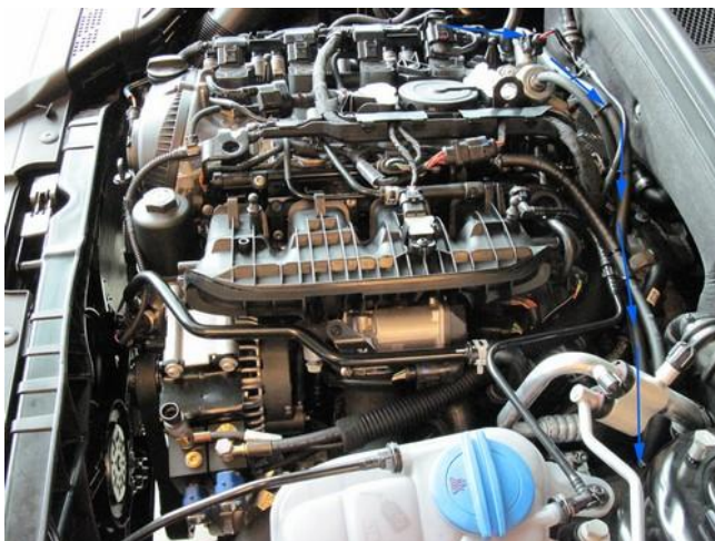
Connect long fuel hose to the just fitted quick release adapter, petrol supply connection.
