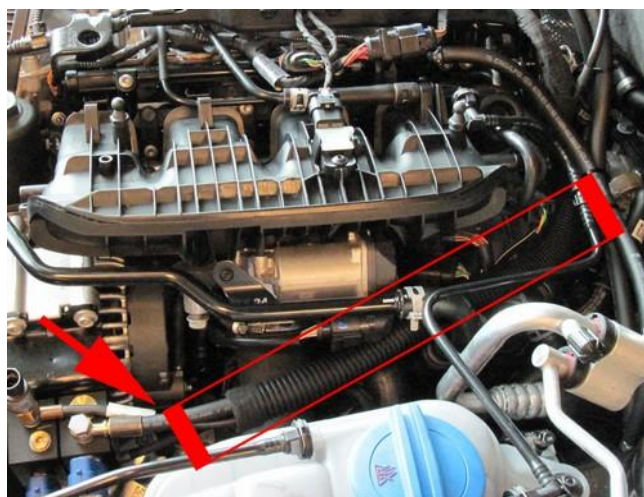
Mount protection tube around the hoses from FSU / FRU to HP pump.
