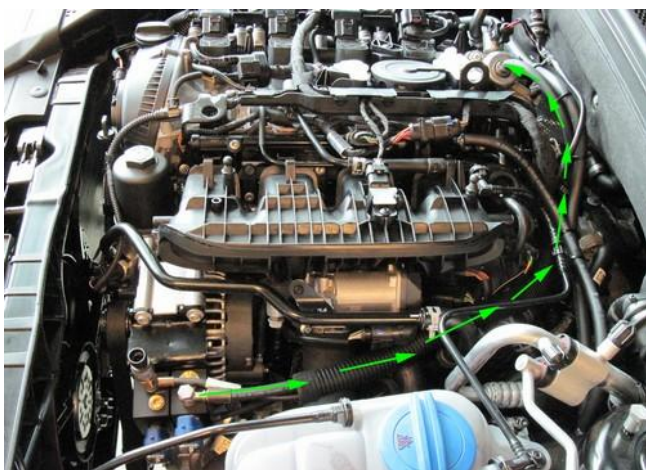
Mount XD-5 hose with banjo bolt to FSU. Mount open end to HPP pump with a 12,8 mm clamp.
