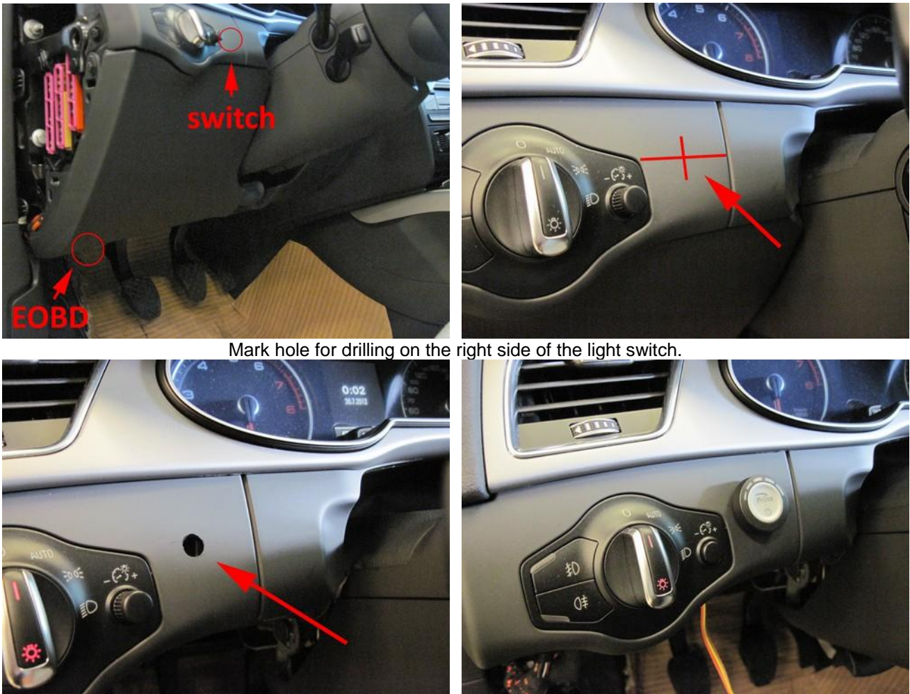
Drill hole Ø8,3mm for mounting switch. Mount switch with the double sided adhesive tape.
