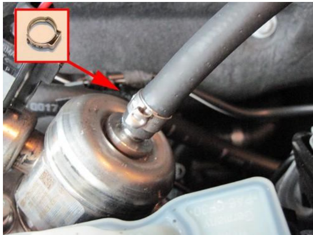
Mount XD-5 hose with banjo bolt to FSU. Mount open end to HPP pump with a 12,8 mm clamp.
