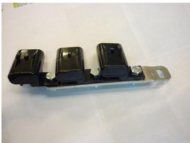
Straighten the fuse bracket.
