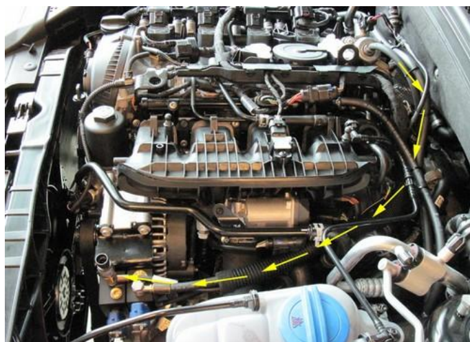
Mount XD-3 hose from HPP pump to FRU. Hose routing.
