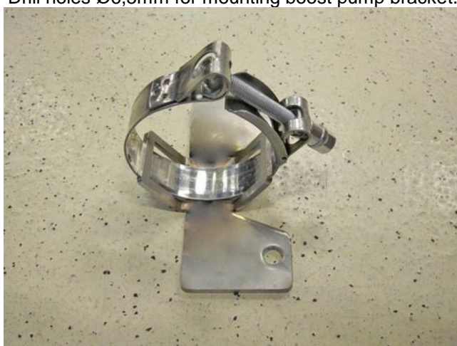
Mount boost pump clamp to bracket.
