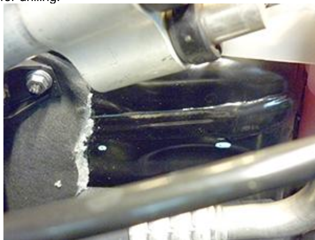
Drill holes Ø6,5mm for mounting boost pump bracket.
