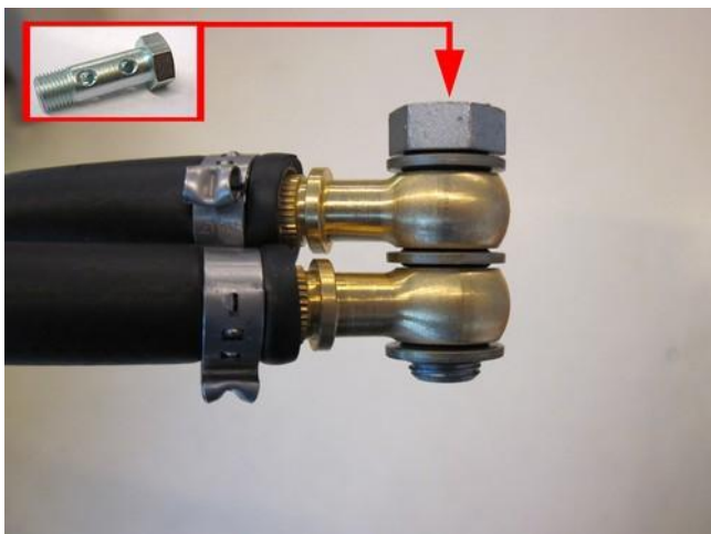
Connect the 2 fuel hoses to the boost pump with a double ( filtered ) banjo bolt.
