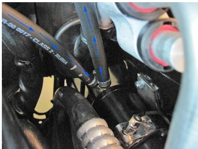
Connect the 2 fuel hoses to the boost pump with a double ( filtered ) banjo bolt.
