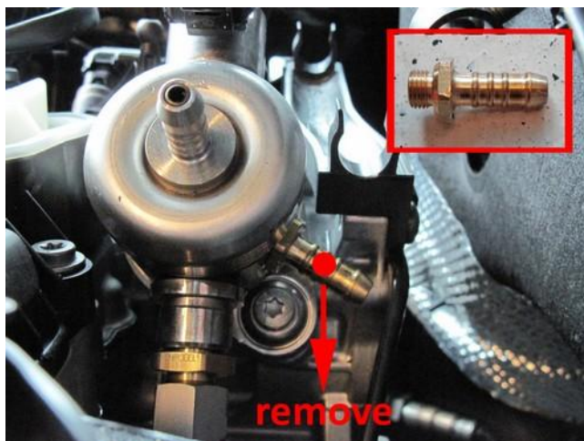
Remove original fuel connection
