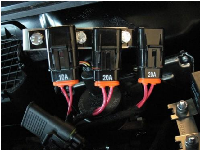
Mount fuse holders to bracket with M6 bolts & spring washers. Mount bracket to threaded rod.
