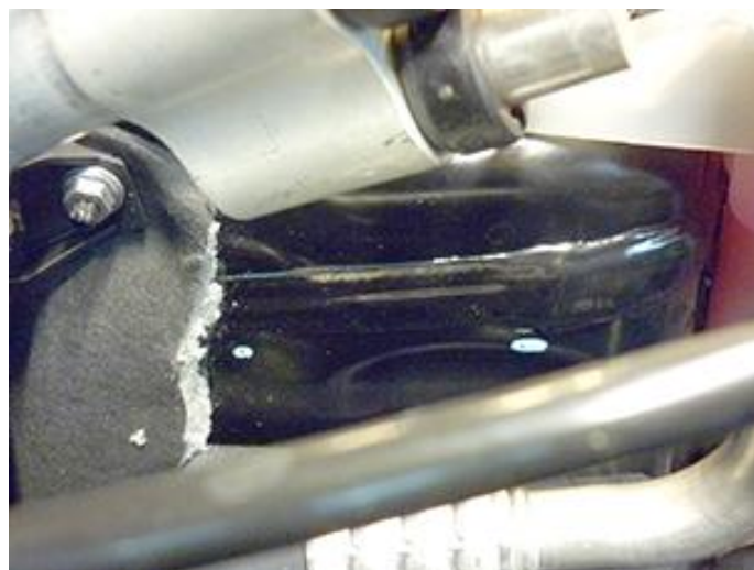
Drill holes \varnothing 6,5\text{mm} for mounting boost pump bracket.
