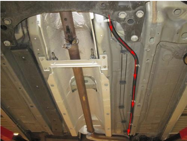
Mount hoses to tank to FSU & FRU. Hose routing.
