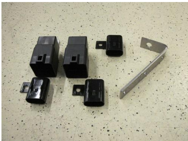
Mount relays and fuse housings to bracket.
