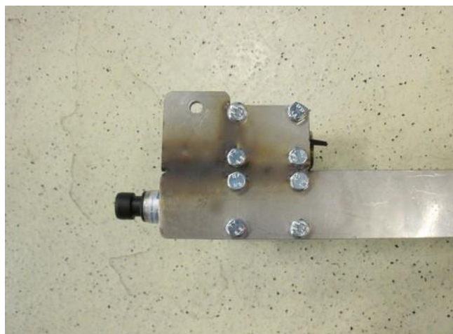
Mount the FSU & FRU on the fuel bracket. Mount bracket with FSU / FRU on original mounting points.
