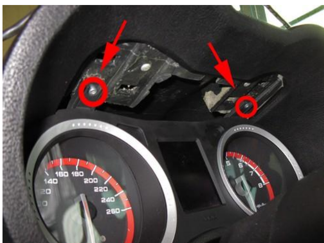
Remove instrument cluster. Connect Wake-up to black connector (see electrical connections)
