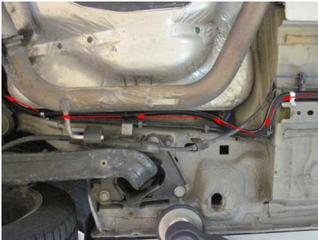
Mount hoses to tank to FSU & FRU. Hose routing.
