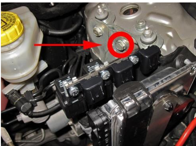
Mount bracket to original bolt on left suspension strut just behind the AFC.
