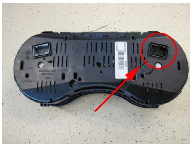
Remove instrument cluster. Connect Wake-up to black connector (see electrical connections)
