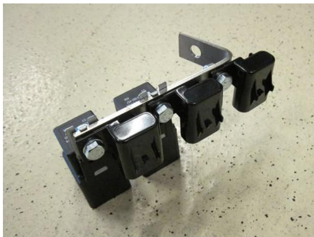
Mount relays and fuse housings to bracket.
