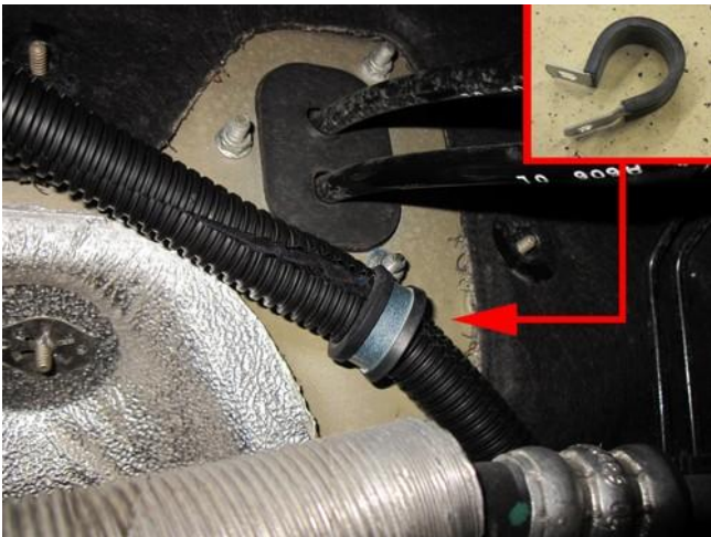
Mount hoses to tank to FSU & FRU. Hose routing.
