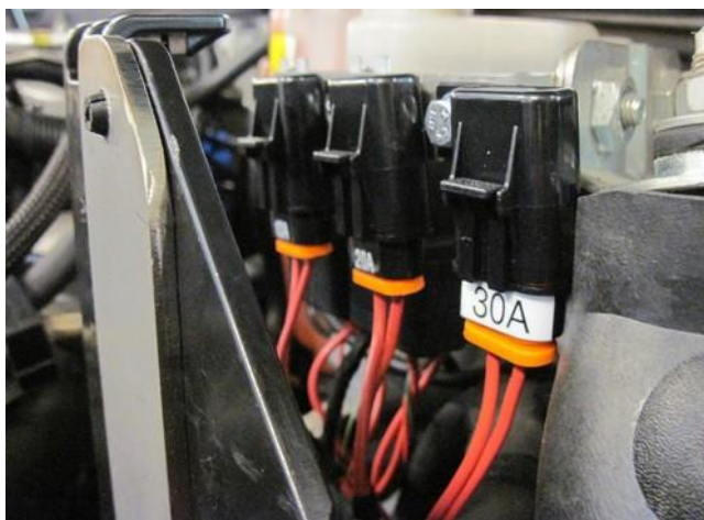
Mount fuses to fuse holders. Also the location for the diagnostic connector (with pull strap).
