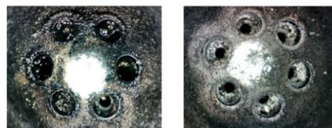
Injector nozzle before cleaning
