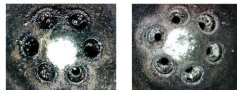
Stop directly when misfire is occurring, in this case Injector must be cleaned outside of the engine. (Ultra sonic cleaning)
