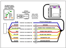
The LPG VSI switch with internal beepers is programmable for different types of tank indicators. Standard setting of the switch is 0-95 Ohm.
